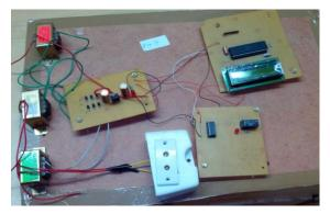
Fig: 3. Picture of Under/Over Frequency Relay
